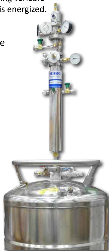
2T DStat Superconducting Magnet Insert installed in standard LHe Storage Dewar
