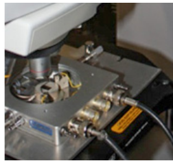
Photograph of the Linkam HFS600E-PB4 probe system in the lab at RMIT, where it is used to apply an oscillating electric field during Surface Enhanced Raman Scattering.
