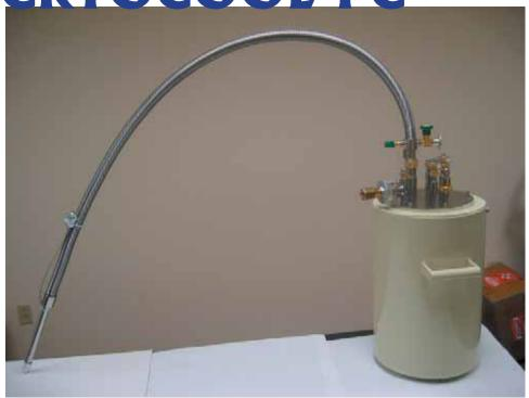
With transfer line for remote cooling
